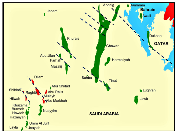
Figure 2- The petroleum fields of Saudi Arabia, Qatar and Bahrain (Husseini, 1995, 1997). Dragging on the southern end of Dukhan field, offset in the middle of Abqaiq and northern Ghawar structures are evident which probably related to rejuvenated Najd Fault zone. The lineaments picked from the topographic maps and Land Sat images in the southern end of Ghawar and Khurais structures could be related to the reactivated Najd Fault System. Tinat, Dilam, Raghbi and Abu Markhah fields are aligned with same fault zone (Perinçek et al., 1998b, 2000a-b).
