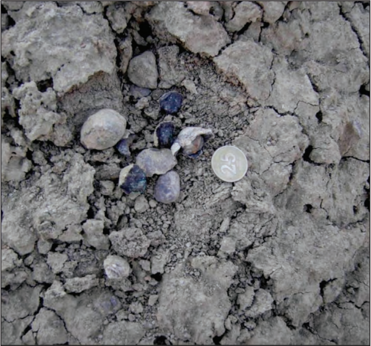
Figure 21- Manganese nodules with copper encountered in claystone and marl of the Koçali complex
