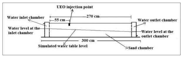
Figure 1- Sideway view (cross section) of the plexiglass tank used for the experiment.
