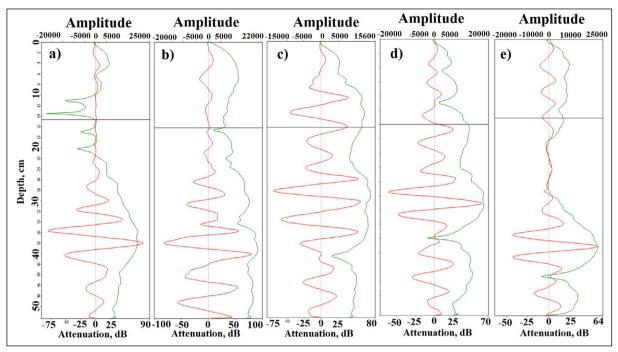
Figure 6- 1D Time-lapse vertical signal amplitude and attenuation graphs at point 50 cm. The black lines show the signal amplitudes and the red lines show the signal attenuations. a), b), c), d) and e) are the radargrams from data before contamination, one hour, 2 weeks, 4 weeks, and 26 weeks after initial contamination, respectively.
