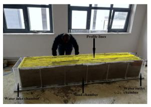
Figure 2- Image of the plexiglass tank showing the three chambers of the tantk and the profile lines (yellow lines).
