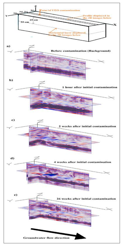
Figure 7- 3D cross sectional time-lapse of GPR radargrams showing the cross section of profile 4 and horizontal layer taken from a depth of 25cm. P1, P4, P5, P8 are the locations of profiles 1, 4, 5 and 8 respectively. a), b), c), d) and e) are the radargrams from data before contamination, one hour, 2 weeks, 4 weeks and 26 weeks after initial contamination, respectively.
