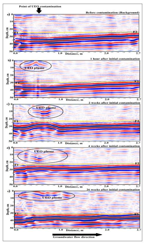
Figure 4 - 2D Time-lapse vertical view of GPR radargrams from profile 5 (XZ plane). The yellow line labelled F1-F2 represents the boundaries between unsaturated and saturated sand, black circles indicate the extensions of the oil plume, a), b), c), d) and e) are the radargrams from data before contamination, one hour, 2 weeks, 4 weeks, and 26 weeks after initial contamination, respectively.
