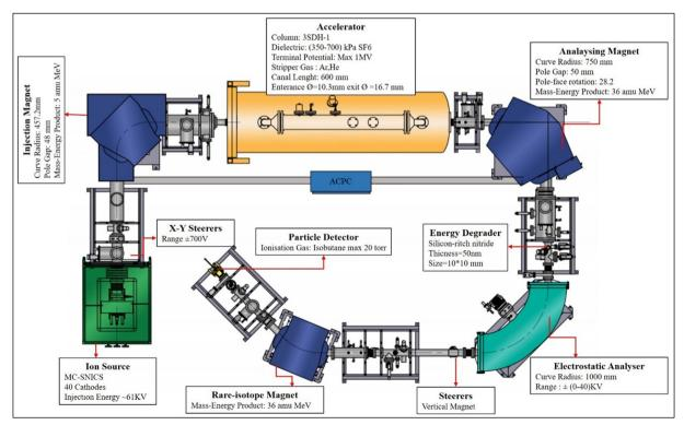
Figure 2- The layout of the 1MV AMS system and the details of the components.
