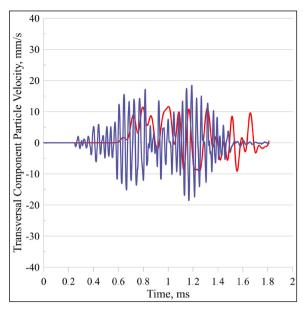
Figure 10- Numerical model predicted (red) and actual blast data (blue) (40 m from the blast).
