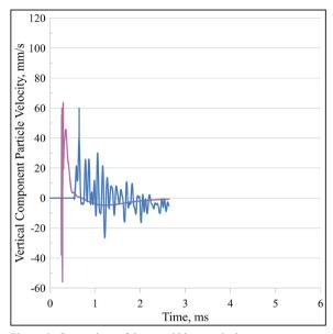
Figure 6- Comparison of the actual blast vertical component source signal and the predicted signal with numerical modeling (purple real data vs blue numerical modeling data).
