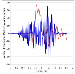
Figure 9- Numerical model predicted (red) and actual blast data (blue) (30 m from the blast).
