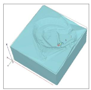
Figure 4- Group and pilot blast and seismograph locations defined in the model. No:1 blast location; No: 2, 3, 4, 5, 6, 7 seismograph locations.
