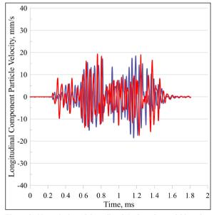
Figure 8- Numerical model predicted (red) and actual blast data (blue) (20 m from the blast).
