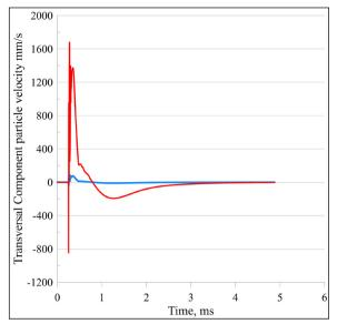
Figure 3- Seismic energy at zero point: The (red) seismic waveform obtained by linear summation of the pilot signal and calculated according to the non-linear behavior (blue). The accepted one is the blue one.
