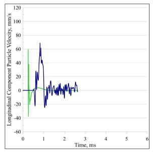
Figure 7- Comparison of actual blast longitudinal component source signal and predicted signal with numerical modeling (green true-blue numerical modeling)
