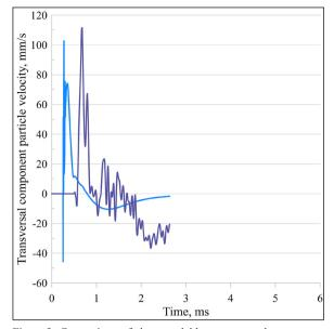
Figure 5- Comparison of the actual blast transversal component source signal and the predicted signal by numerical modeling (light blue real data vs dark blue numerical modeling data).
