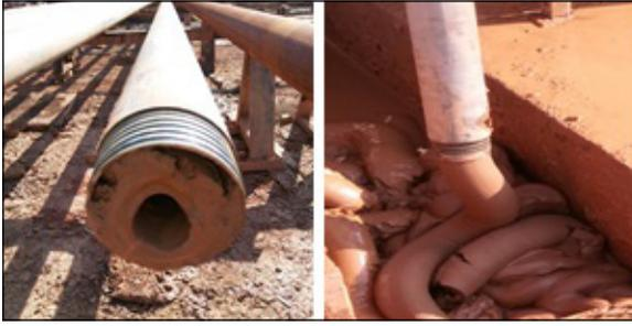
Figure 5- The in-pipe caking and the rate of caking seen during the cleaning of the inside of the pipe.
