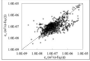
Figure 10- The comparison between c<sub>v</sub> values calculated from Equation 3 and 4.
