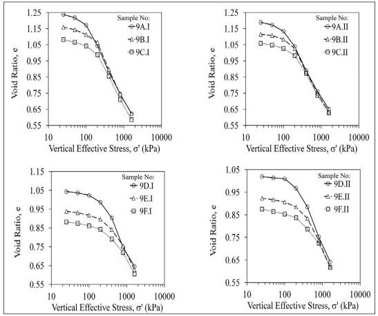
Figure 2-  $e-\sigma$ ' curves obtained from conventional oedometer tests.
