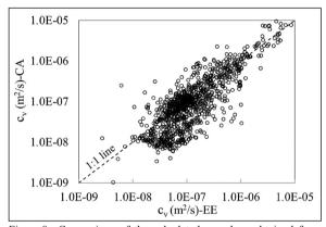
Figure 8- Comparison of the calculated  $c_v$  values obtained from the empirical equation and the combined apparatus (EE: empirical equation, CA: combined apparatus).
