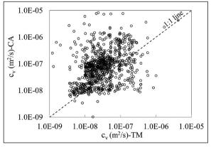
Figure 9- Comparison of the calculated c<sub>v</sub> values obtained from the Taylor's t<sub>90</sub> method and the combined apparatus (TM: Taylor's t<sub>90</sub> method, CA: combined apparatus).
