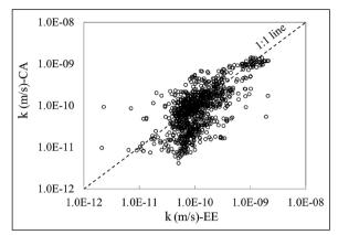
Figure 7- Comparison of the k values obtained from the empirical equation and the combined apparatus (EE: empirical equation, CA: combined apparatus).
