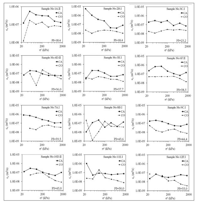
Figure 5- Changes in the cv values with increases in load levels (CA: combined apparatus, CO: conventional 1D oedometer).
