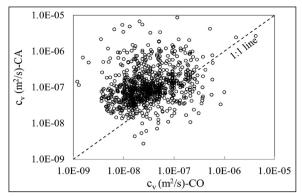
Figure 6- Comparison of c<sub>v</sub> values obtained from the combined apparatus and conventional 1D oedometer (CO: conventional oedometer, CA: combined apparatus).
